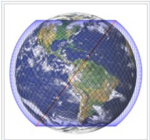
The Starlink constellation, phase 1, first orbital shell: 72 orbits with 22 each, therefore 1584 satellites at 550 km (350 miles) altitude
