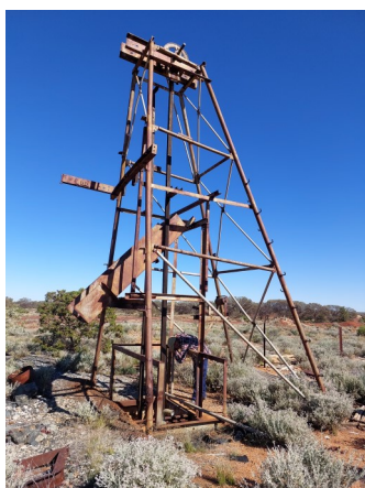
The headframe of the old Pelerin mine now Aurumins ground—within a historically high gold production area
